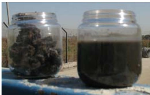
20 cu.m of sludge can be dewatered to 15-30% dry solids daily in one press requiring only a single phase power supply
