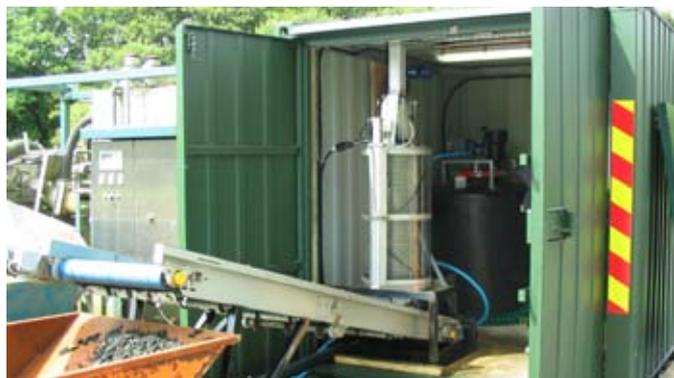
Containerised, single or multiple, ASP presses with conveyors provide flexible fixed or mobile sludge dewatering capability.
