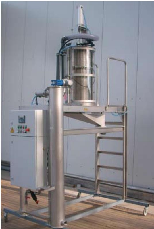
The Cequesta ASP Automatic Sludge-dewatering Press offers a simple and economic alternative to existing dewatering systems for small to medium capacity water and wastewater treatment plants. Unlike traditional systems, the Cequesta ASP has few moving parts and consumes very little energy. Moreover, this innovative and well-proven dewatering solution employs a fully automated batch-treatment approach, requiring little human intervention.
