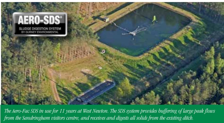
*The Aero-Fac SDS in use for 11 years at West Newton. The SDS system provides buffering of large peak flows from the Sandringham visitors centre, and receives and digests all solids from the existing ditch.*
