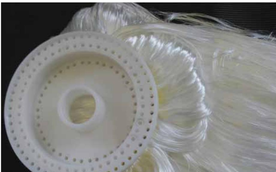
*The unique VPMF fibre media provides filtering from 0.2 micron up to 25 micron when in the fully compressed filtering mode, but relaxes during backwash to easily and quickly release contaminants.*
